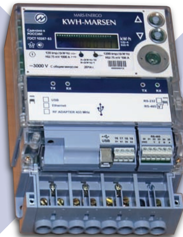
2-channel KWH-Marsen with internal Voltage Divider 3 kV Overall dimensions (height × width × depth): 277 × 170 × 83 mm, or less Weight: 1.5 kg, or less.
